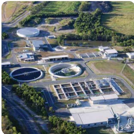
Alliance for the construction of a new 17MLD STP, and a new 12MLD recycled water plant (with 9MLD installed membrane capacity). The project also includes 2 years of operational support and optimisation.
